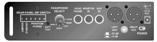
HEADPHONE SELECT: Selects which signal is being sent to the Headphone Output as well as the front panel meters; Stereo, Mono, Right, Left, or the Monitor signal.
