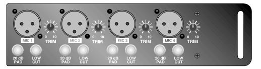
MIC 1 - 4: Balanced XLR connectors for connection to dynamic or condenser microphones. +48 volts of phantom power is available for each input.
