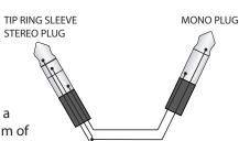
Tip and Ring are wired together, then connected to the Tip of the Mono Plug.
