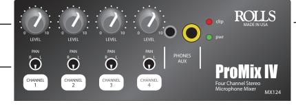
Clip LED: Indicates that clipping is about to occur or occurring in the MX124 circuitry. This LED begins to light 3dB below actual circuit clipping.
